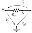
$$V_{dd} - V_{\gamma} - V_{2} = 0 \longrightarrow V_{2} = i_{2}R_{2} = V_{dd} - V_{\gamma} \longrightarrow i_{2} = \frac{V_{dd} - V_{\gamma}}{R_{2}} = \frac{24 - 0.7}{2} = 11,65 \text{ mA}$$
