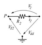
$$V_{Z2} + V_{dd} - V_2 = 0 \longrightarrow V_2 = i_2 R_2 = V_{Z2} + V_{dd}$$
